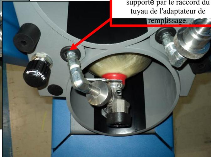
Figure 2 – Remplissage incorrect
